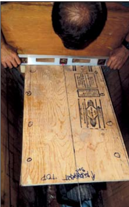
(left) Checking shaft position with laser level. (right) Engine mockup in position to locate engine beds. On this engine, the mid-point of the adjustable engine mounts lined up almost exactly with the gearbox output flange. If they were lower, we would have had to make a wooden support at each end of the plywood to position the reference wire.
