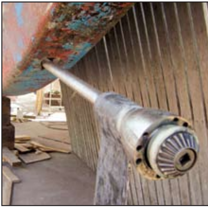
Propeller shaft initial fitting and marking for strut.
