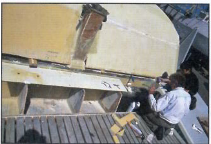
New fuel tank being installed in locker.
