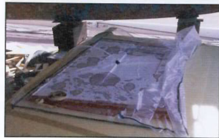
(top) A panel under vacuum. The red fabric is peel ply; the quilted white polyester breather/bleeder material is on top. (bottom) Another flat panel under vacuum. The excess resin is coming through the laminate stack and is being absorbed by the breather/bleeder material.
