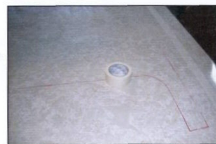
Mold table with outline of a panel written on the table with indelible marker to act as a cutting template for fiberglass fabric and other vacuum bagging consumables.
