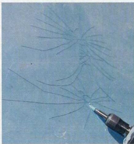
Photo 1: Cut a shallow V in a gelcoat crack with a Dremel tool and a grinding attachment
