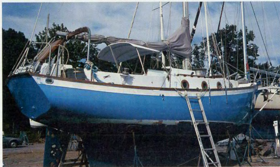
Photo 5: The author's boat, with three coats of one-part polyurethane paint applied
