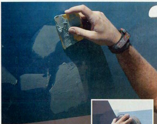
Photos 2–3: Spread the filler evenly over voids and overfill so the dry surface can be sanded smooth
