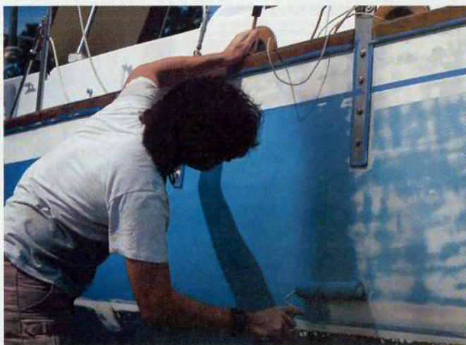
Photo 4: Roll on the finish paint over the primer (here finely sanded), then tip off with a brush to ensure a smooth surface
